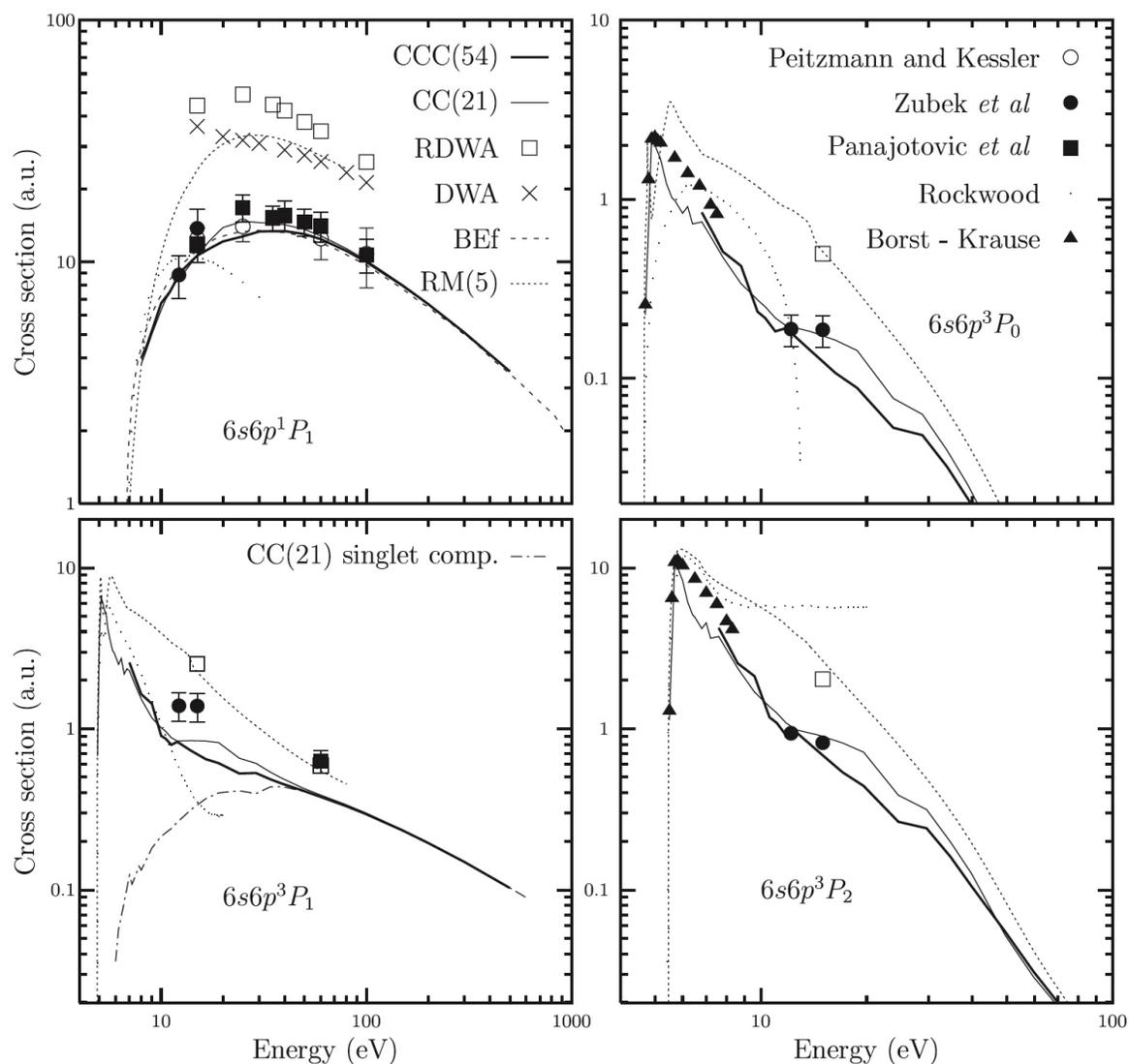
**Figure 9.** Electron-impact ICs for the  $6s6p^1P_1$  and  $6s6p^3P_{0,1,2}$  states of mercury from the ground state. Theory and experiment are as in figure 3. In addition, RM(5) calculations are due to Bartschat (2002), BEf results are due to Kim (2001) and the experimental data for the  $6s6p^3P_{0,2}$  states are due to Borst (1969) and Krause *et al* (1977).
