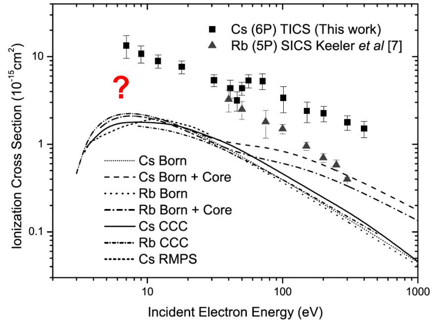
FIG. 6. The measured TICS out of the Cs  $6^2P_{3/2}$  state compared to SICS from CCC, RMPS and Born calculations. For comparison, the results of our CCC, and Born SICS calculations for Rb  $5^2P$  state are also compared to the SICS data of Keeler *et al.* [7].
