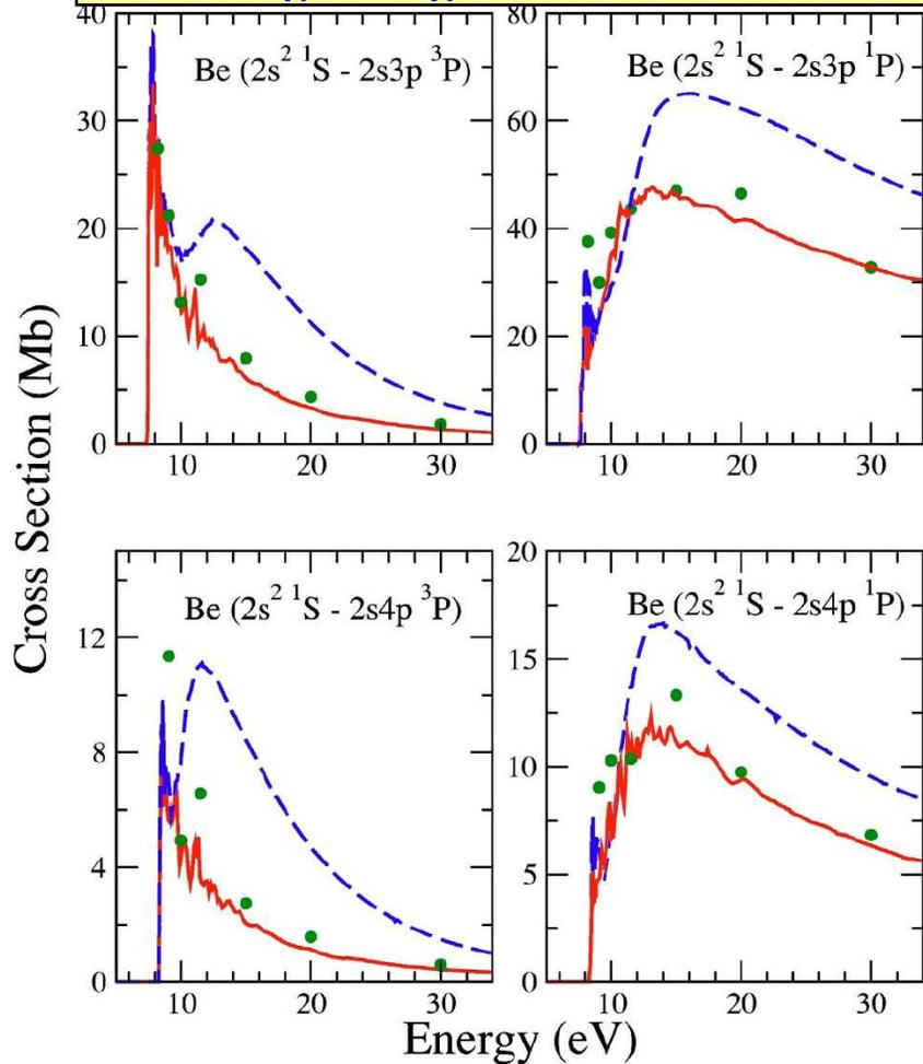
FIG. 2. Electron-impact excitation cross sections from the  $2s^2 1S$  ground term of Be to the  $2snp^3P$  and  $2snp^1P$  excited terms for  $n=3$  and 4. Dashed curves are from the present 29-term *R*-matrix calculation; solid curves are from the present 280-term RMPS calculation; solid circles are from CCC calculations as described in Fursa and Bray [10] and provided at the CCC database web site [11].
