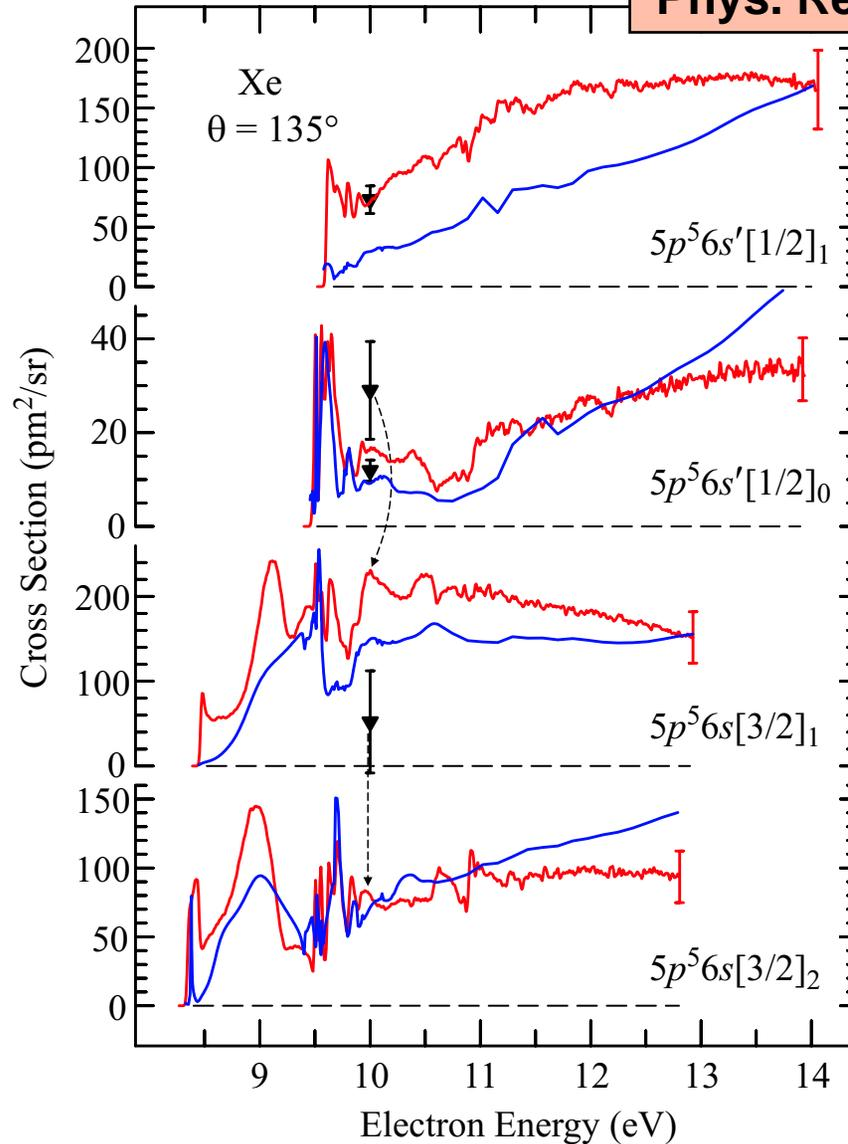
Angle-differential cross sections for electron-impact excitation of the lowest four states of xenon as a function of impact energy at a fixed scattering angle of  $135^\circ$ .
