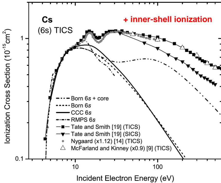
FIG. 4. Experimental TICS from the Cs ground state, rescaled to CCC and RMPS calculated SICS between 4–10 eV, as discussed in the text. The Born SICS also show the contribution from  $5p$  and  $5s$  core ionization, with calculated threshold energies of 22.9 and 38.0 eV, respectively. Tate and Smith’s [19] rescaled SICS is also shown, indicating the contribution to the TICS from multiple ionization.
