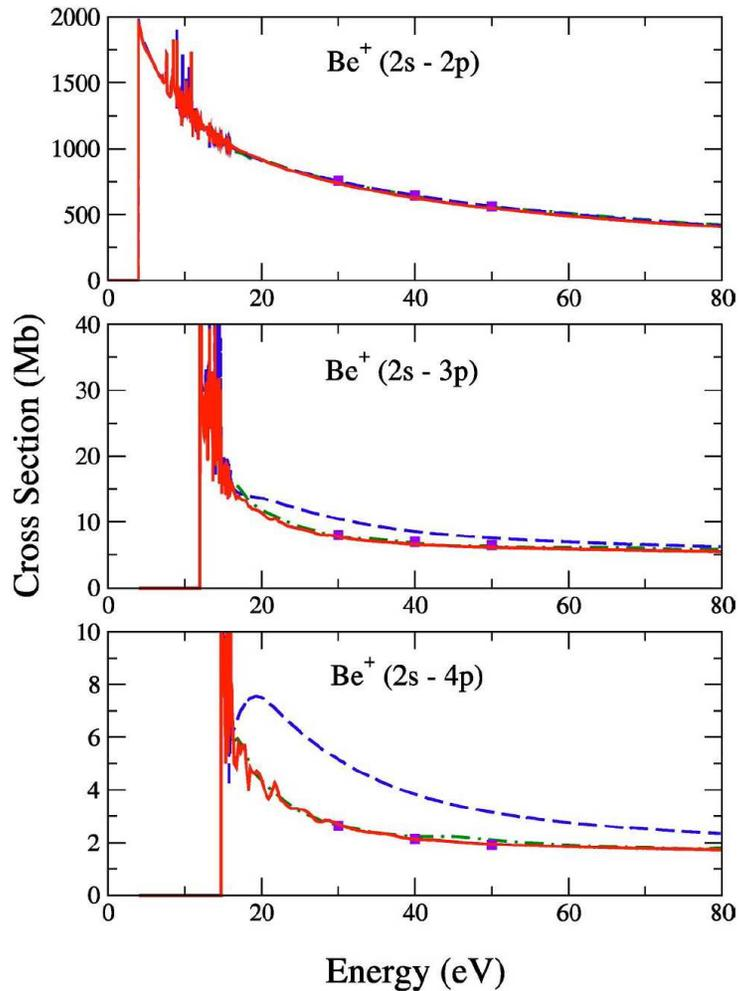
FIG. 4. Electron-impact excitation cross sections from the  $2s$  ground term of  $\text{Be}^+$  to the  $np$  excited terms. Dashed curves are from the present 14-term  $R$ -matrix calculation; solid curves are from the present 49-term RMPS calculation; solid squares are from the present TDCC calculation; dot-dashed curves from the CCC calculation by Bartschat and Bray [14].
