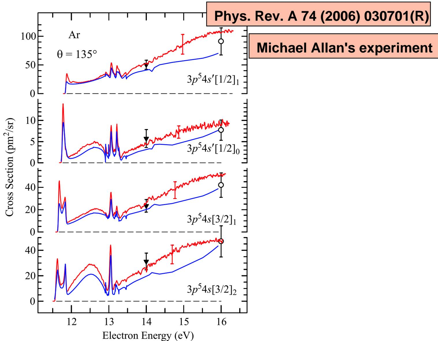
Angle-differential cross sections for electron-impact excitation of the lowest four states of argon as a function of impact energy at a fixed scattering angle of  $135^\circ$ .
