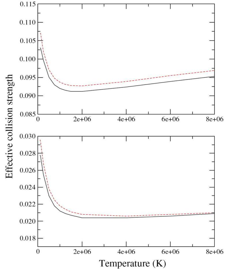
**Figure 2.** Effective collision strengths for two double-electron transitions; results from the Breit–Pauli *R*-matrix calculation are represented by the solid lines and those from the Dirac *R*-matrix calculation by the dashed lines. The upper graph is for the  $3s^2\ ^1S_0-3p^2\ ^1D_2$  transition and the lower graph is for the  $3s^2\ ^1S_0-3p^2\ ^3P_2$  transition.
