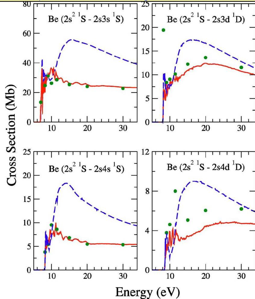
FIG. 3. Electron-impact excitation cross sections from the  $2s^2 1S$  ground term of Be to the  $2sns^1S$  and  $2snd^1D$  excited terms. Dashed curves are from the present 29-term *R*-matrix calculation; solid curves are from the present 280-term RMPS calculation; solid circles are from CCC calculations as described in Fursa and Bray [10] and provided at the CCC database web site [11].
