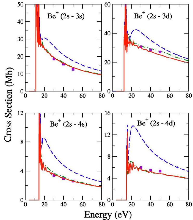
FIG. 5. Electron-impact excitation cross sections from the  $2s$  ground term of  $\text{Be}^+$  to the  $ns$  and  $nd$  excited terms. Dashed curves are from the present 14-term  $R$ -matrix calculation; solid curves are from the present 49-term RMPS calculation; solid squares are from the present TDCC calculation; dot-dashed curves from the CCC calculation by Bartschat and Bray [14].
